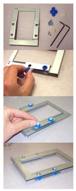
**STEP 4:** Align the bracket on the hard drive as shown. The ends of the four screws should align with the holes in your hard drive. Be sure to orient the drive and bracket as shown in the picture: The hard drive's IDE and power connections should be at the end of the bracket with the L-shaped bend.
