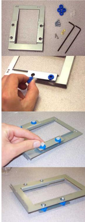
**STEP 4:** Align the bracket on the hard drive as shown. The ends of the four screws should align with the holes in your hard drive. Be sure to orient the drive and bracket as shown in the picture: The hard drive's IDE and power connections should be at the end of the bracket with the L-shaped bend.
