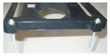
Insert two plastic spacers onto each of the two screws, and use a nut to keep the spacers in place. You can hand-tighten the nut at this stage.
