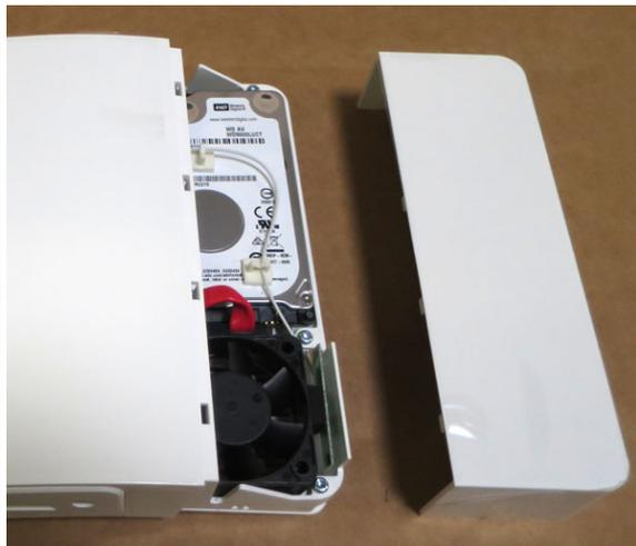
Figure 6 – Removing side lid
