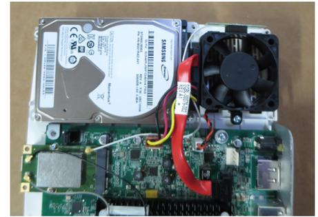
Figure 14 – Drive installed
