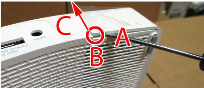
Figure 5 - Removing side lid
