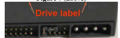
Two-jumper Maxtor Set as “Master”
